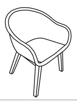
Turn chair upright. Assembly is now complete and chair is ready for use. Ensure all bolts are fully tightened every 3 months to ensure stability.
