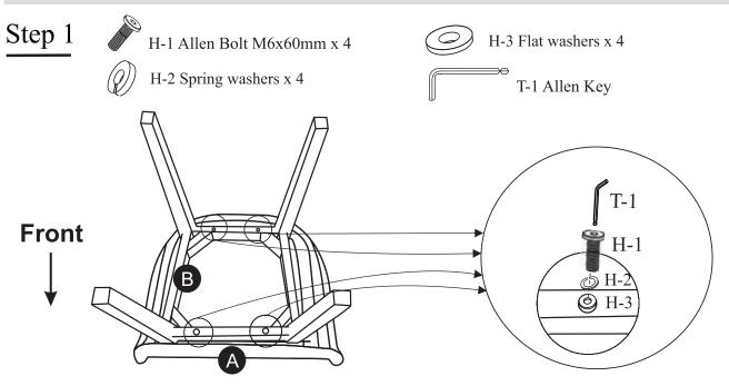
Place Seat (A) upside down on a padded, non-marring surface. Position Leg Assembly (B) upside down onto Seat (A) and align all mounting holes. Secure Leg Assembly (B) to Seat (A) with Allen bolts (H-1), Spring Washers (H-2) and Flat Washers (H-3) using provided Allen Key (T-1), stacking the hardware in the order as shown. Engage all hardware first, then fully tighten. Do not over tighten.
